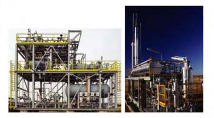
The TEG Regeneration process typically consists of a still column, an overhead condenser, and a reboiler where the rich glycol thermally regenerated to remove excess water and to regain the high purity to pumped back to the top of the Contactor Tower to repeat the process after passing through the Flash Drum and Filters to remove scaling and dissolved hydrocarbon.
